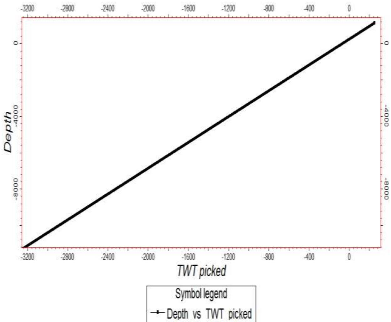
Time (Figure 4 ) and depth structural contour maps were produced for the two horizons defined on top of sand bodies, namely, Horizon A and B. Both types of structural contour maps show similar structural relationship. This linear relationship was also corroborated by the linear curve
