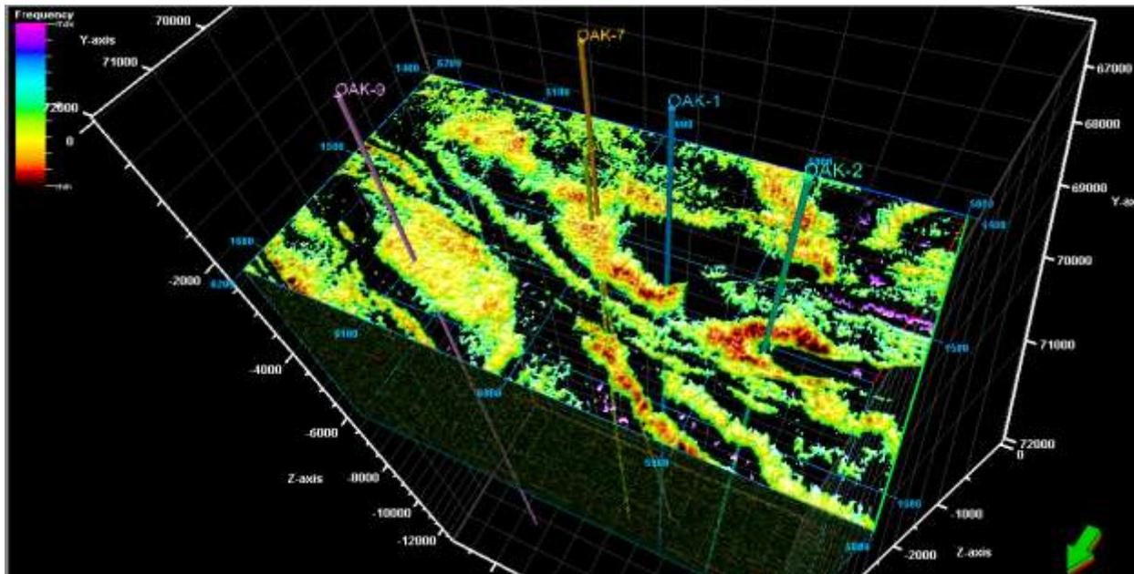
Figure 3: Frequency Attribute Model showing Sand body in Reservoir A and B.
