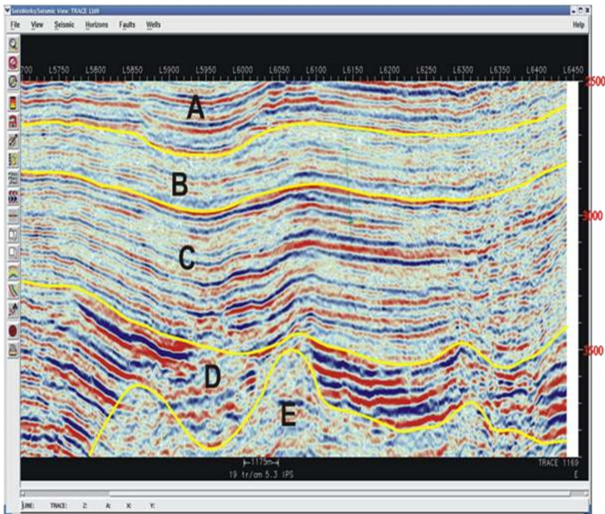
Figure 4 : Seismic reflection attributes in terms of seismic packages
