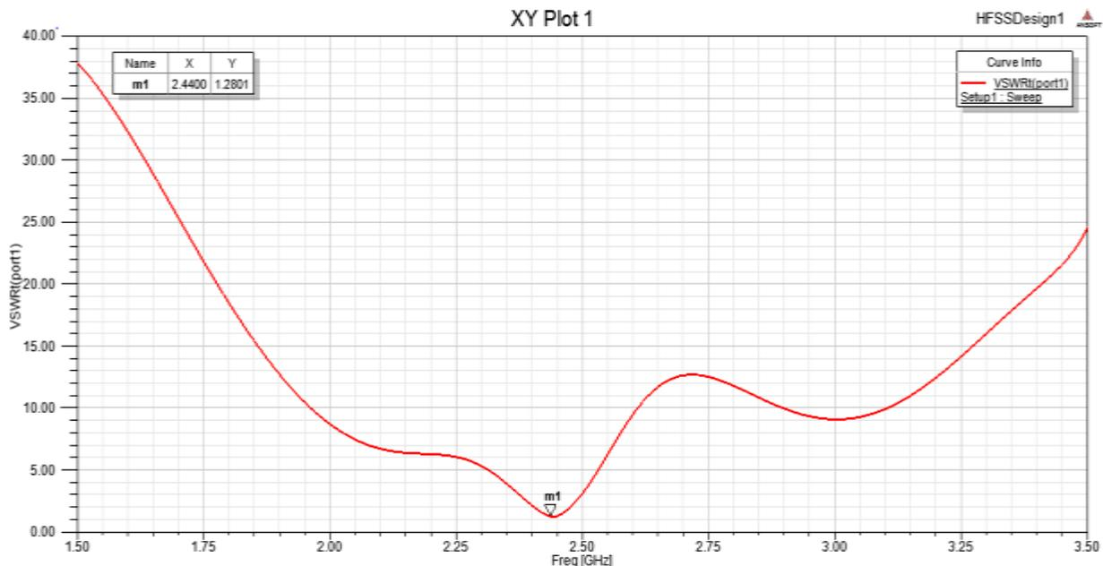
**Figure 10.** VSWR plot Here the value for the proposed microstrip patch antenna was 1.2801 at the resonating frequency of 2.44GHz.
