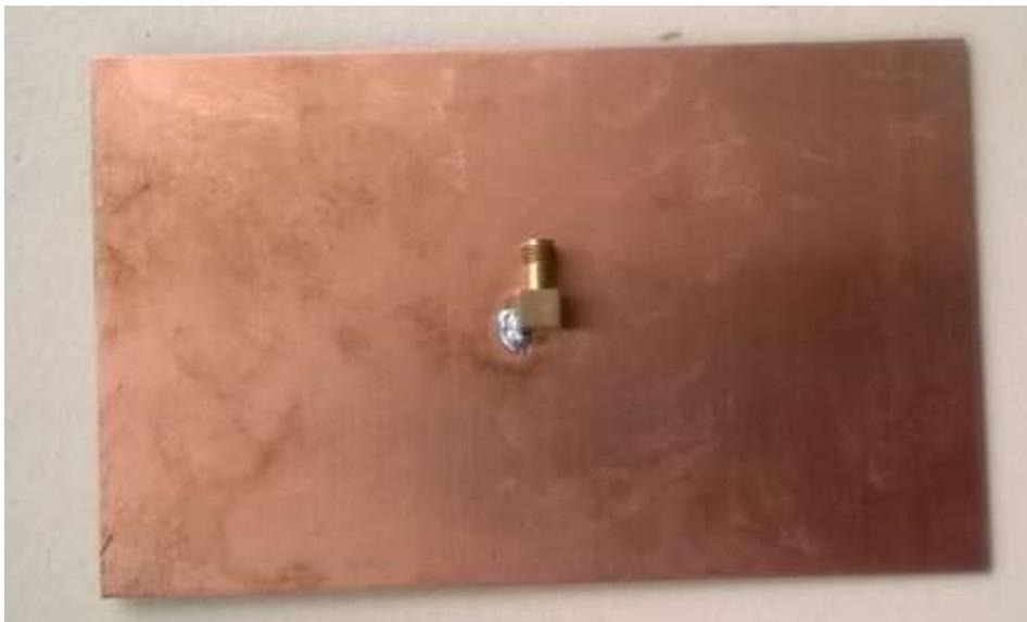
Figure 4. Ground plane of the patch antenna array
