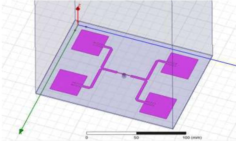
**Figure 1.** 4 element patch antenna HFSS model
