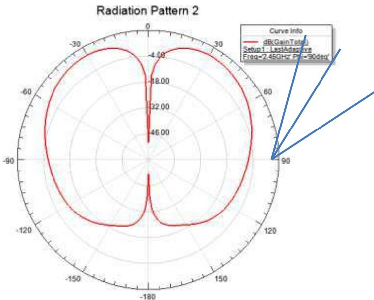
**Figure 7.** Simulated H-plane ( $\theta=90^\circ$ ,  $\phi$  varying)
