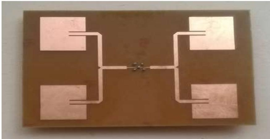
Figure3. Implemented 4-element patch antenna array
