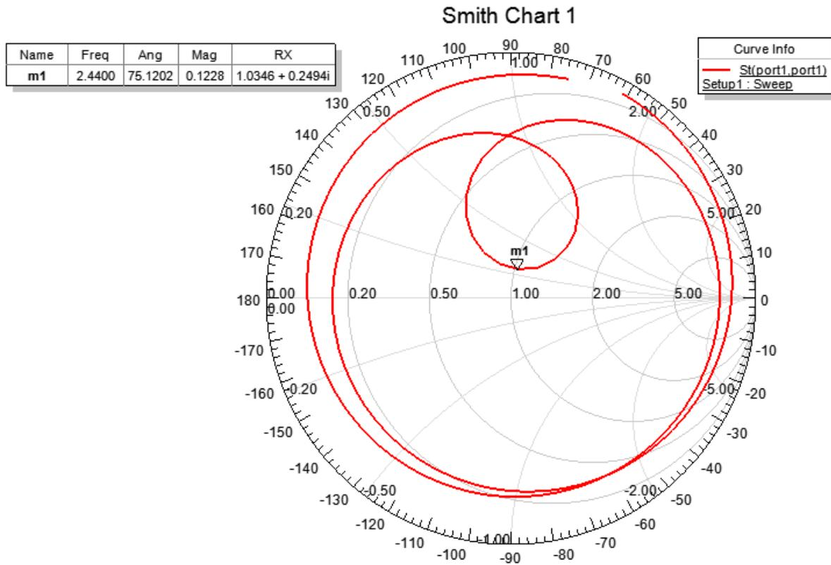
Figure 11. Smith chart of the proposed patch antenna
