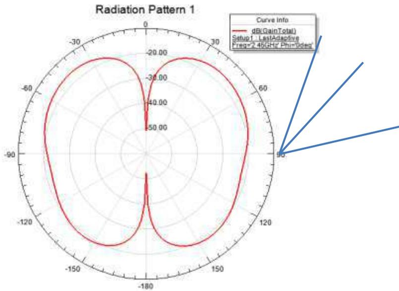
**Figure 6.** Simulated E-Plane ( $\phi=90^\circ$ ,  $\theta$  varying)
