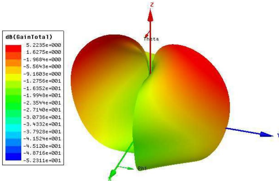
**Figure 8.** 3D radiation pattern
