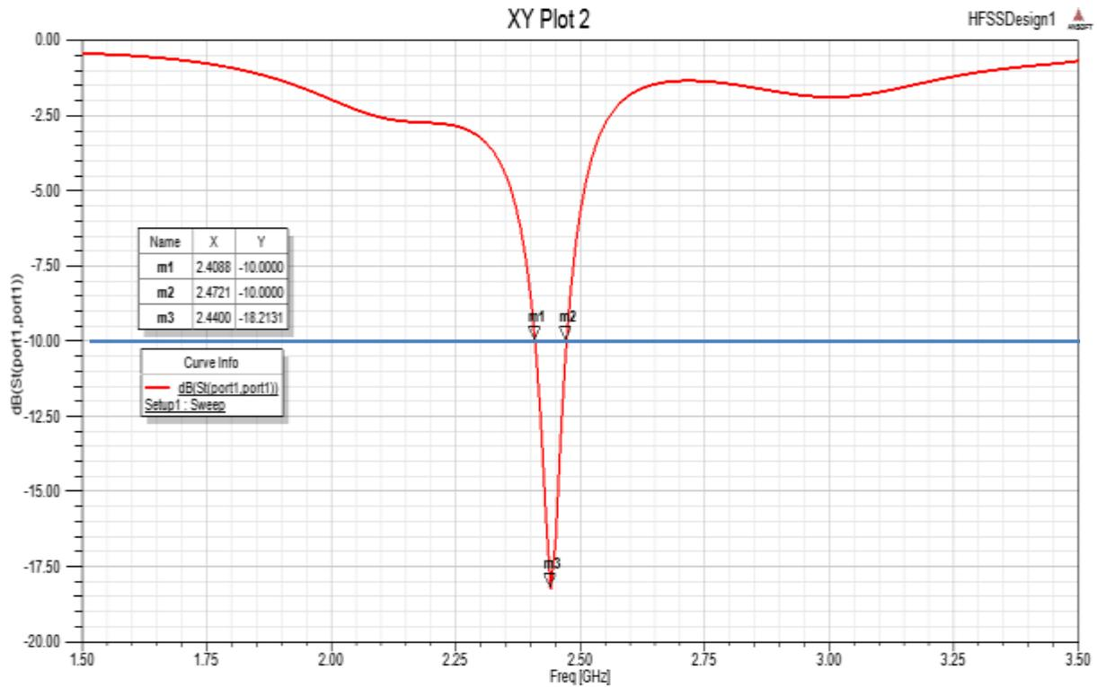
**Figure 5.** Return loss  $S_{11}$  obtained for the patch array
