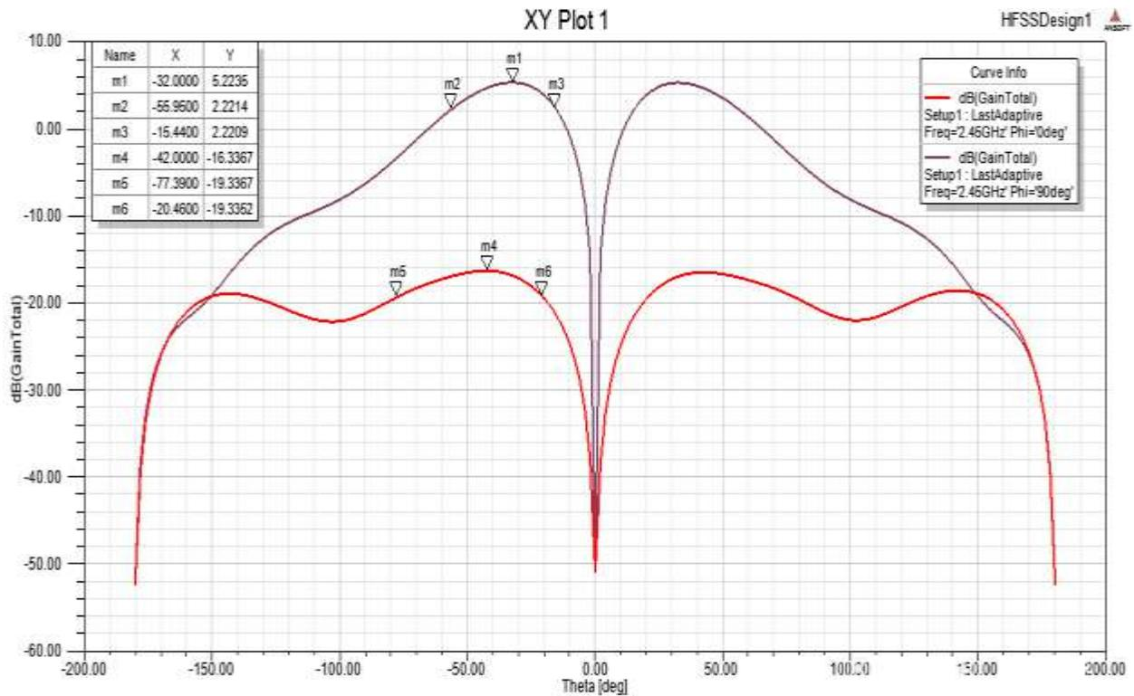
**Figure 9.** E-Plane and H-Plane patterns in rectangular coordinates
