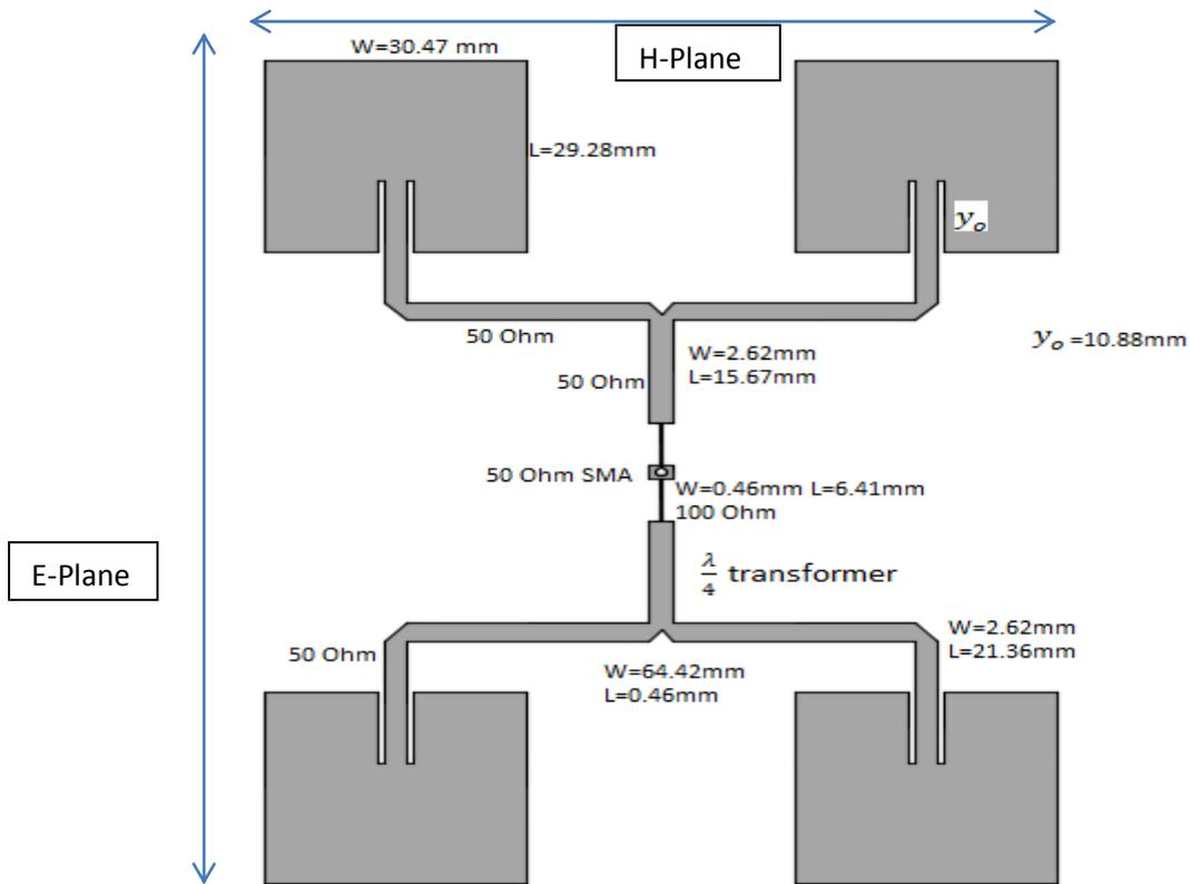
**Figure 2.** 4-element patch antenna PCB layout with dimensions
